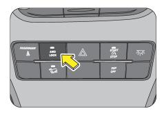
In an AWD vehicle, power is transmitted to all the wheels. This is managed by the AWD System which intelligently transfers torque to all four wheels. AWD system includes electromagnetically operated clutch which is controlled by an ECU. According to the driving conditions this system automatically delivers torque to the rear wheels.
