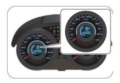
The odometer records and displays the total distance traveled in kms. Press the reset button (A) to cycle through odometer and tripmeter displays. Odometer cannot be reset.
