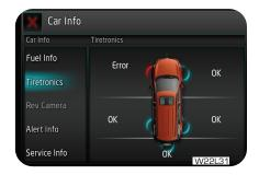
Examples of Tiretronics warning lamp illumination and corresponding infotainment screen display;
