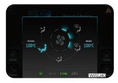
Air is discharged through the foot/floor vents on the instrument panel.
