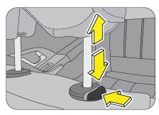
Always align top of the head restraint with the top of your head or as close to it as possible. To raise the head restraint, press the lock knob and pull the restraint up. To lower the head restraint, press the lock knob and push the head restraint down.
