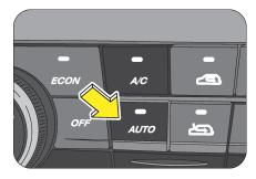
The auto mode can be used to control the complete air conditioning operation of the vehicle automatically. The auto mode controls blower fan speeds, air intake mode, temperature and modes (vents) based on the set temperature.
