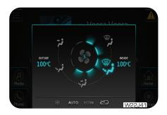
Air is discharged through the foot/floor vents, windshield vents and side defrost vents on the instrument panel.
