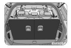
Access to or exit from third row seat and luggage area is possible by completely folding the second row seat. Second row seat features 60:40 split configuration. Instead of folding the complete seat back and seat cushion, the required seat alone can be folded to gain access to third row seat.
