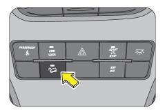
Assists the driver to descend a steep hill (max 50% inclination) by means of brake intervention limiting the vehicle speed is without driver's input.
