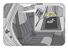
To change the second row seat back angle, lean forward slightly while raising the recline lever on the top corner of the seat back, lean back to the desired position and release the recline lever. Make sure the recline lever returns to its original position and the seat back is locked in place by rocking the seat back forward/backward.
