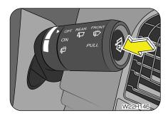
The auto wipe feature works by sensing water (by the RLS) on the windshield. Based on this input, the wipers are turned ON/OFF. For Eg., this feature will be helpful when the rain is inconsistent.
