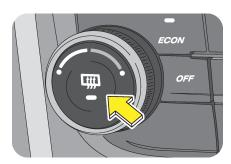
Rear windshield glass defogger switch is located on the temperature control dial in the central switch bank. Press the switch once to activate the defogger. The lamp on the switch illuminates upon activation and the defogger heats the rear windshield clearing the fog/ frost.
