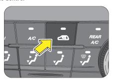
To set the HVAC system to fresh air mode, press the re-circulation mode button again. The LED on this button switches OFF, indicating that re-circulation mode is active.
