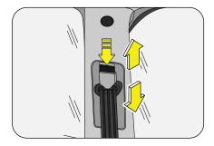
You can adjust the height of the shoulder belt anchor for maximum comfort and safety in both front seats. If the height of the seat belt is too near your neck, you will not be getting the most effective protection. The shoulder portion of the belt should be adjusted so
