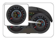
When coolant temperature reaches the red zone, the high engine coolant temperature warning lamp illuminates.
