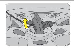
To remove the wheel cover, wrap the tip of a screw driver with cloth, insert it near the lugs of the wheel cover and pry the cover away from the wheel.
