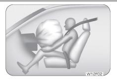
Front airbags are not intended to deploy in side-impact, rear impact or rollover crashes. In addition, front airbags will not deploy in frontal crashes which are below the prescribed deployment threshold where risk of serious injuries is low.
