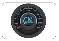
The speedometer indicates the real time road surface speed of the vehicle in kilometers per hour.
