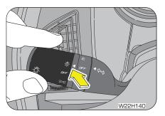
To turn ON the auto head lamp feature, rotate the outer rotary switch on the lighting control stalk anti-clockwise aligning the "arrow" on the stalk to the auto head lamp icon on the switch. This is indicated by the auto head lamp tell tale in the infotainment screen.
