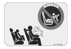
Never place a rear-facing child restraint in the front passenger's seat. If the airbag deploys, injuries to the child may be fatal..
