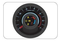
The tachometer indicates the real time engine speed in thousands of RPM (revolutions per minute). Each division is 500 RPM. Running the engine in very high RPM leads to excessive engine wear and poor fuel economy. Maintain steady engine speed below 2500 RPM and do not accelerate or decelerate abruptly.
