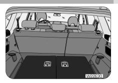
To fold the third row seat, unlock the seat back by pulling the lever on the rear of the seat back outwards.
