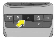
The hazard warning flasher button is located in the central bezel switch bank. Press the button to turn ON the hazard warning flashers, all directional turn signals will flash to warn oncoming traffic. This is an emergency warning system and should be used only when there is an emergency. Use it when your vehicle is disabled and is a safety hazard for other motorists. Hazard warning flasher will work in all positions of the ignition key and even when the vehicle is fully locked.
